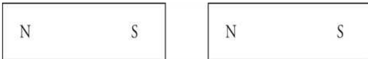
Cutting the bar magnet in half just gives you two smaller bar magnets. You can never get an isolated north or south pole.
